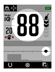
The Target ID number on the Detect Screen, showing detection of a US quarter with a Target ID of 88.
