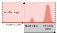
If the Threshold Level is just right, it should sound like a faint audible hum. This emphasises variations in signal response making targets easier to hear.
