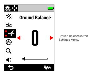
The default Ground Balance setting of O (zero) is recommended for All-Terrain modes because these locations typically have less mineralisation than gold prospecting locations.
