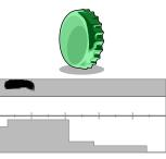
Bottle cap B laid on edge (vertical). In this case the detector sees very little of the flat shape of the object, and the response lies in the upper ferrous region.
