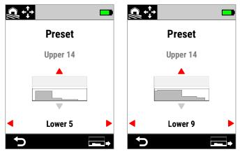
The Lower Limits Preset increased from 5 to 9 by pressing  $\blacktriangleright$  .
