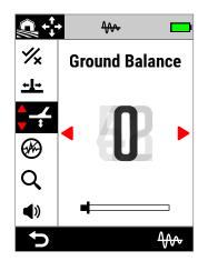
The Ground Balance value will update automatically as it tracks to changing ground conditions.
