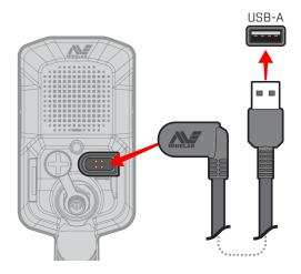
**3.** The green Charge Status LED on the top left of the Control Pod will flash slowly. When the battery is fully charged, the Charge Status LED will remain On.
