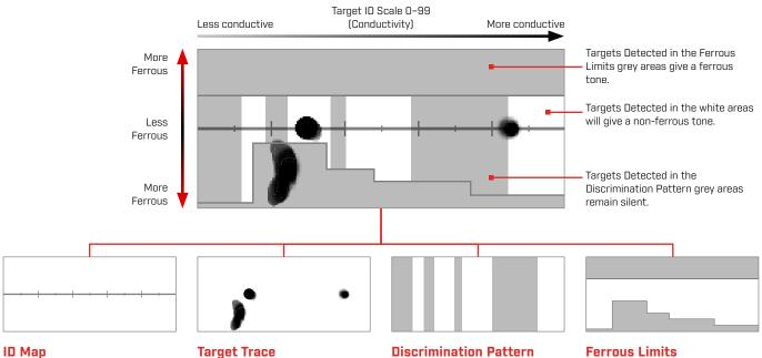
The ID Map has a conductive horizontal axis and ferrous vertical axis.
