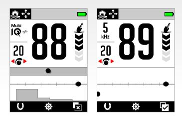
This example shows the detection of a coin and a nail in Multi-IQ+, then again using a single frequency. While the coin's Trace and ID remain very similar, the ferrous nail appears on the far lower left when in a single frequency.
