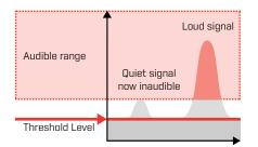
If the Threshold Level is too low, the variation caused by a small or deep target may be inaudible.
