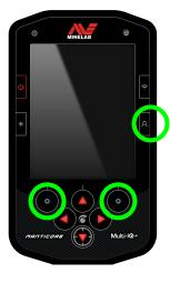
The **Side Soft Key** is the bottom right Side Button on the Control Pod. Actions assigned to it do not display an icon until the Soft Key is pressed.
