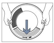
Agitate the contents of the pan by jiggling the pan from side to side, making sure the material doesn't slop out. Do not use a circular swirling motion.
