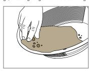
As the material in the pan becomes finer, swish the pan gently through the water and slightly tilt the pan to help the water carry the top layers of silt and sand away.
