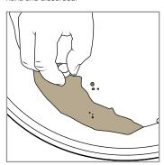
Seal the iron separator magnet in a small plastic bag before you pick up the black sand. When you remove the magnet, you simply need to rinse the bag to discard the unwanted sand
