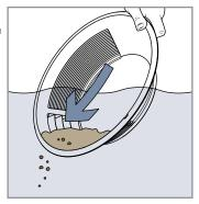
Repeat steps 3 to 5, progressing through the panning zones until the material has reduced significantly, leaving behind a concentrate of fine silt, tiny pebbles, black sand and gold.
