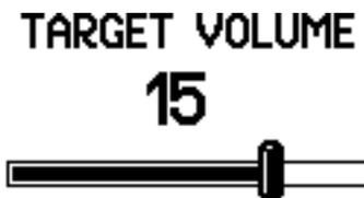
Target Volume can be used to prevent signals from large and shallow items producing very loud signals that are uncomfortable to your ears. This should be adjusted to suit your individual hearing.
