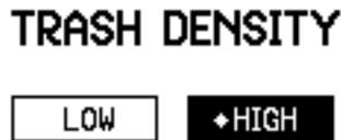
**High** is the factory preset setting, suitable for most common locations where coins and relics are found, and also areas with variable ground mineralisation. The High setting detects targets at a faster rate, so in areas with a lot of trash, particularly if close together, the High setting is more likely to detect the presence of a “good” target in amongst a number of rejected or trash targets.
