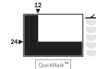
QuickMask™ has two slider controls to adjust the level of Ferrous and Conductivity discrimination.
