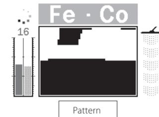
Target information is presented to you via the Smartfind™ Discrimination Pattern, Sensitivity Gauge, FE-CO numbers and Depth Gauge.
