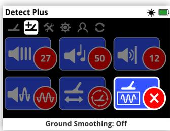
The Ground Smoothing function is located on the Detect Plus page. The Ground Smoothing function has three settings to choose from to suit your detecting requirements.
