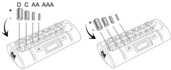
Figure 4 - Insert Batteries from Left to Right
