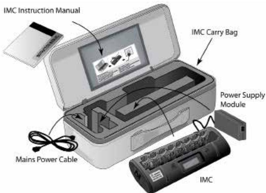
Figure 2 - Parts for the IMC
