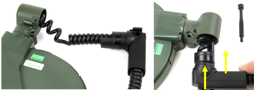
Figure 62: Fitting Pivot Lower Shaft
