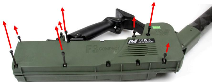
Figure 12: Removing Eight Screws (Allen Key)
