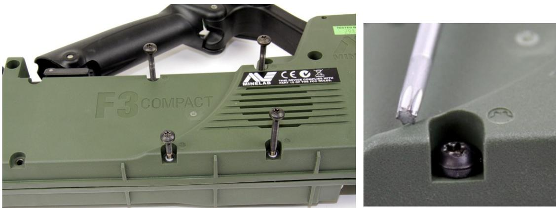
Figure 13: Removing Four Torx Screws
