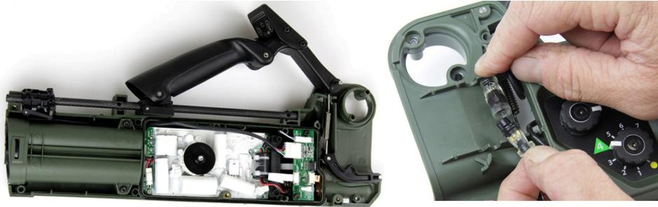
Figure 80: Disconnect Wiring Loom Handle
