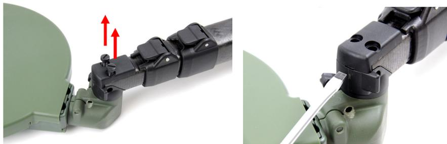
Figure 76: Removing Screws from Lower Shaft
