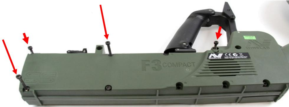
Figure 23: Fitting Four Screws
