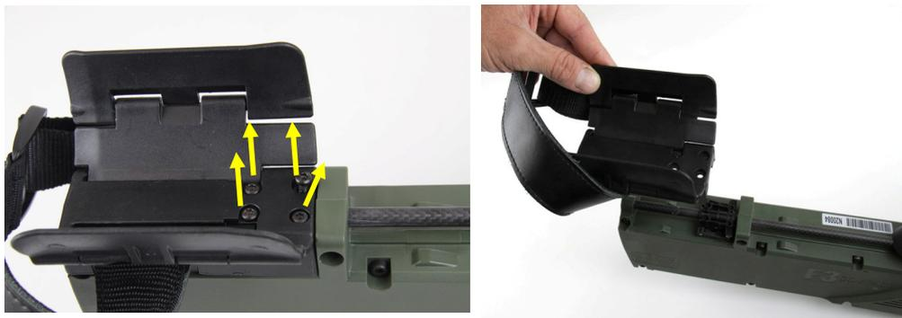
Figure 9: Removing the Armrest
