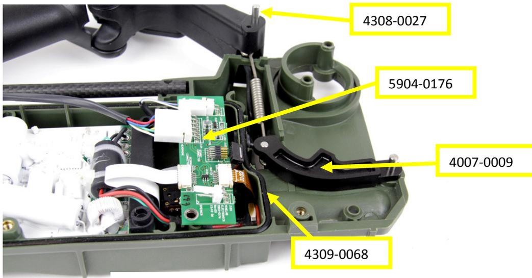
Figure 103: Detector body
