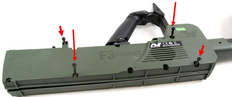
Figure 22: Fitting Four Screws
