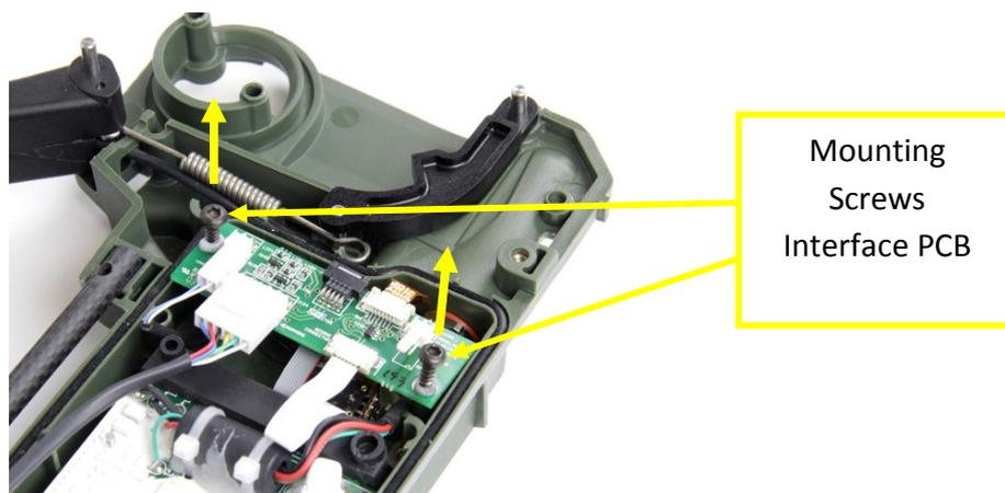
Figure 34: Interface PCB
