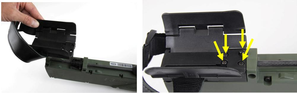
Figure 28: Attaching the Armrest
