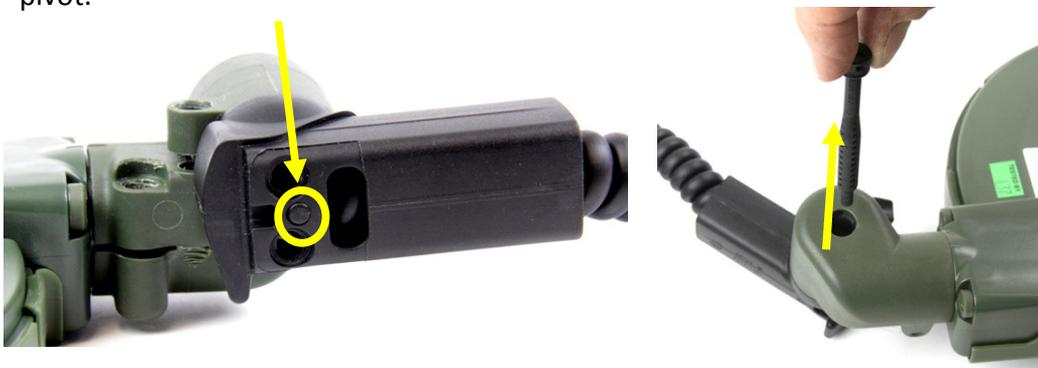
Figure 57: Removing Pin Coil Pivot
