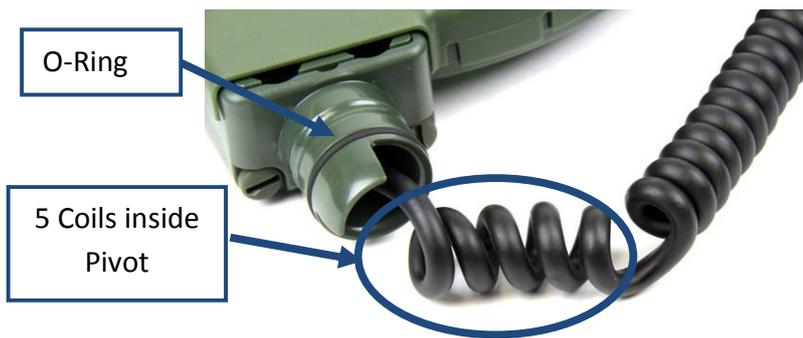
Figure 60: O-Ring and Coil Cable
