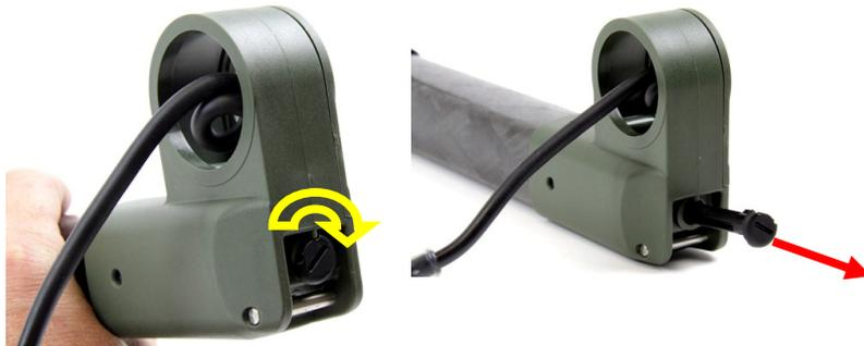
Figure 75: Removing Pin Coil Cable
