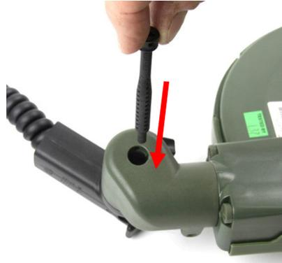
Figure 63: Inserting Pin Coil Pivot
