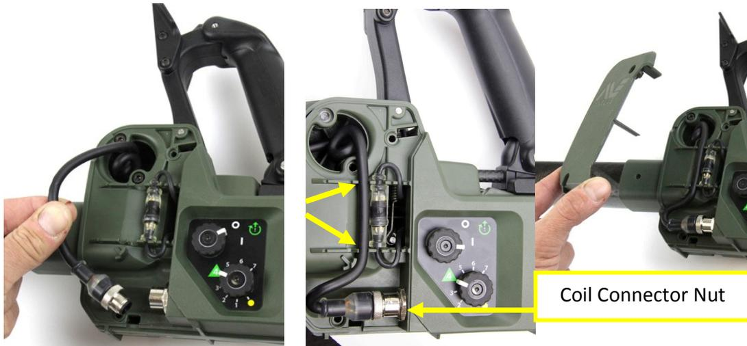
Figure 18: Connecting Coil Cable and Removing Hinge Cover
