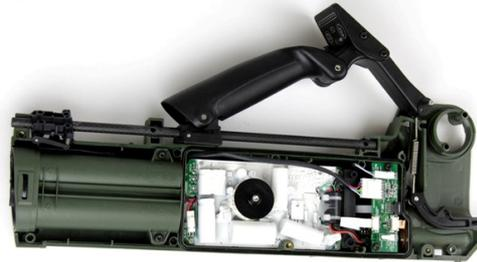
Figure 89: Opened Detector Body
