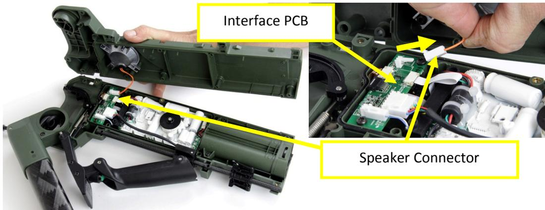
*Figure 14: Disconnecting Speaker Connector*
