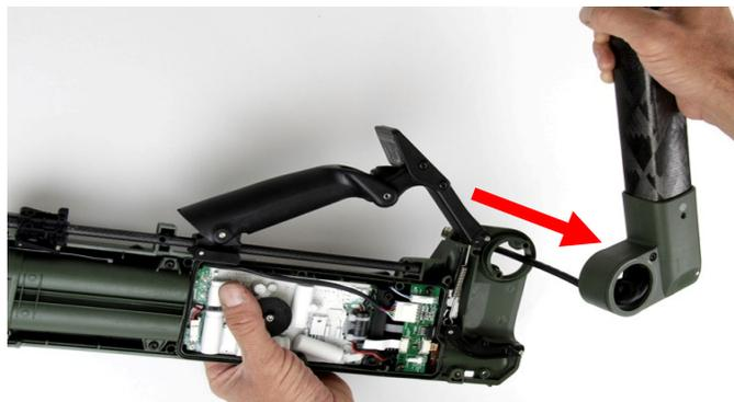
*Figure 15: Removing Shafts*
