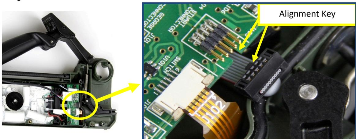
Figure 43: Connector 10 Way
