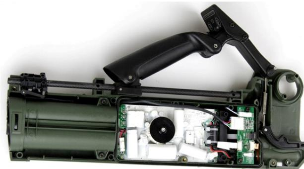
Figure 31: Opened Detector Body
