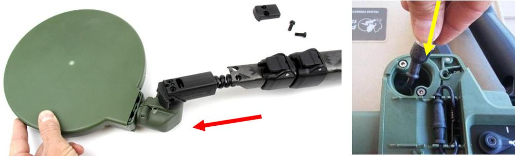
Figure 53: Sliding the Coil Off the Shaft
