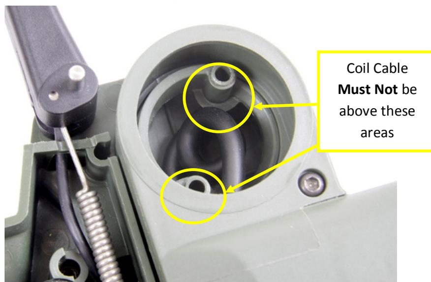
*Figure 21: Coil Cable Position in Shaft Hinge*
