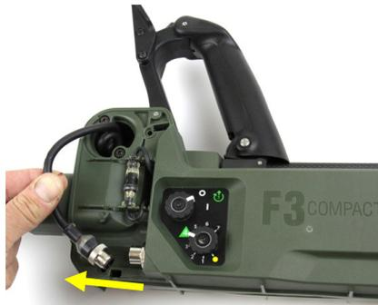
Figure 50: Disconnecting Coil Connector
