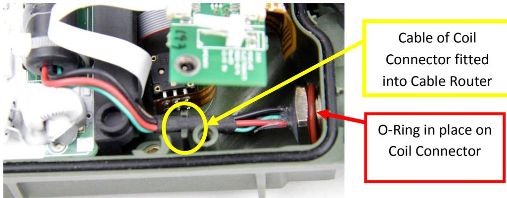
Figure 41: Coil Connector
