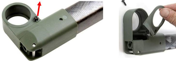
Figure 65: Removing Cover Shaft Hinge
