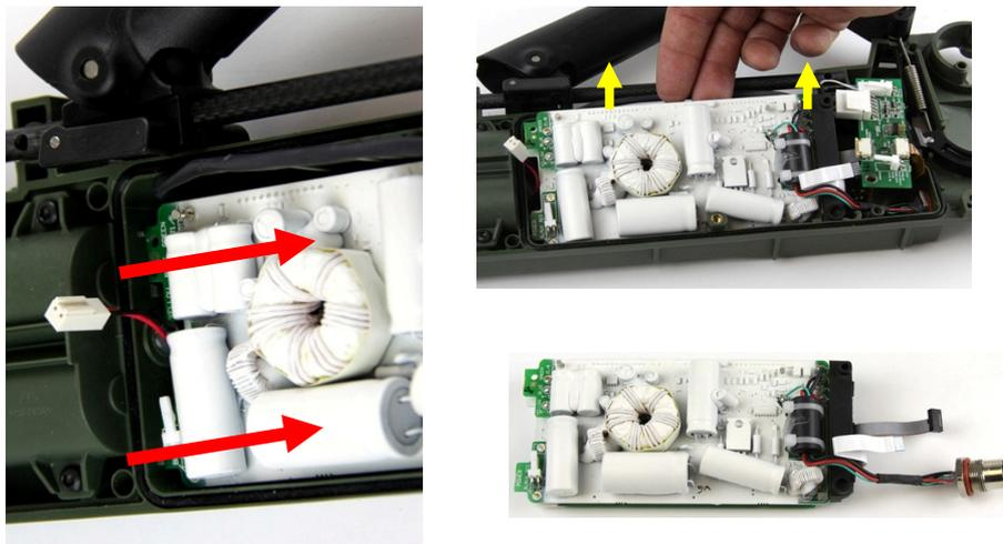
Figure 36: Lifting Main PCB Out of Detector
