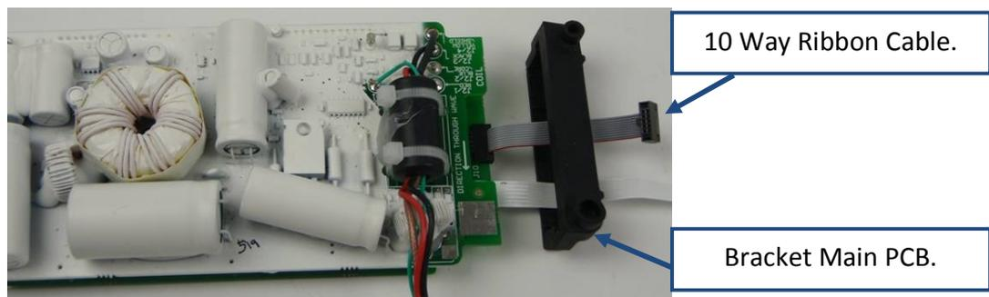
Figure 38: Fitting Bracket
