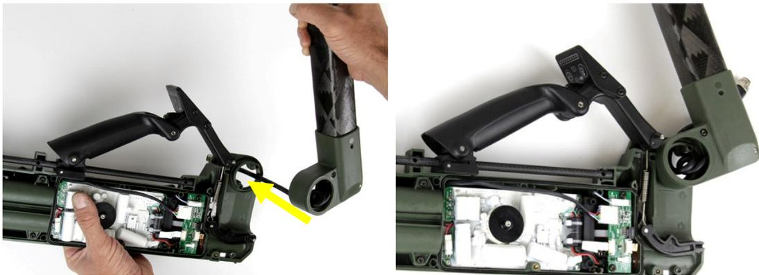
Figure 17: Threading Coil Cable and Attaching Shafts
