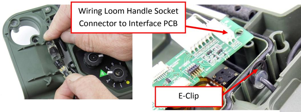
Figure 99: Wiring Loom Handle Socket
