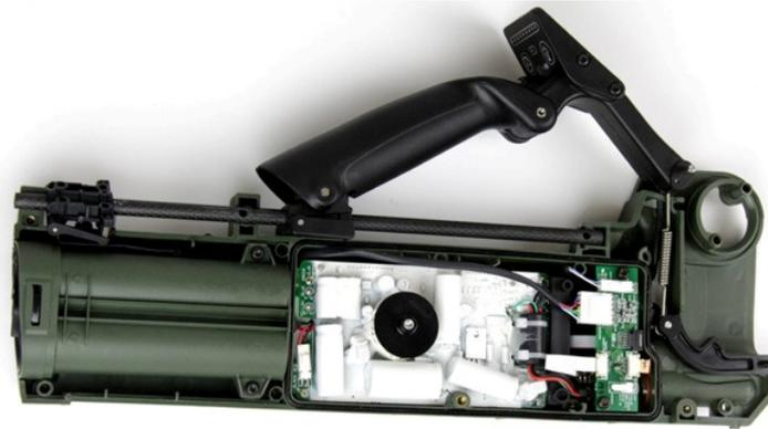
Figure 16: Open Detector Body
