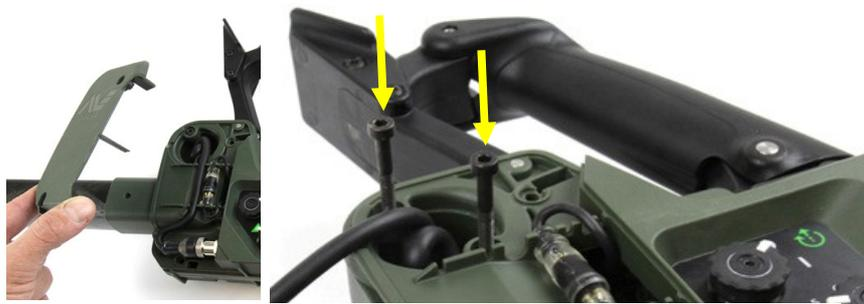
Figure 25: Fitting Screws into the Shaft Hinge
