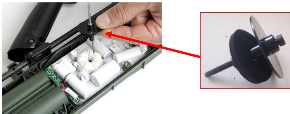
Figure 42: Screw Toroid
