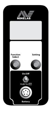
The On/Off switch is located on the Rear Control Panel
