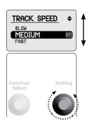
With a function highlighted turn the **Setting** control to the left or right to adjust the setting.
