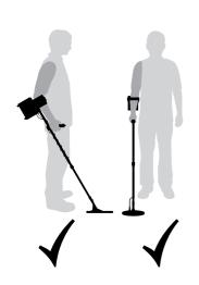
Tip: Some operators may find it more comfortable to fit the battery around the waist. However, make sure the detector isn't detecting a signal from the battery. If using a large coil, position the battery as high up on your back as practical (and comfortable) to avoid any unwanted interference.
