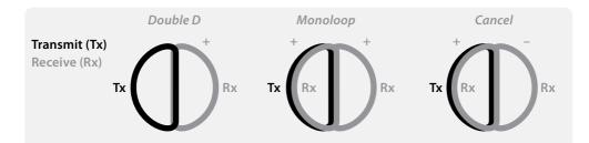
This diagram is a view of the internal coil windings, showing the different receive characteristics of the three Coil/Rx switch options.
