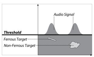
Target signals when detecting in All Metal.
