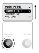
Turn the **Function Select** control left to scroll up the list. The currently selected function is highlighted.
