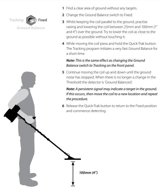
**Note:** Use this procedure to periodically test that you are effectively compensating for ground noise.
