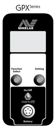
**LCD** (Liquid Crystal Display) Displays all the menu functions and settings. Now with backlight (p. 50).
