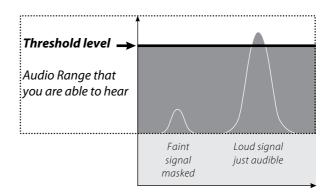
With the Threshold set correctly both target signals are easily heard.
