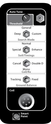
Auto Tune (p. 32) automatically scans a range of frequency channels to help reduce electrical interference.
