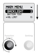
Turn the **Function Select** control right to scroll down the list. The currently selected function is highlighted.
