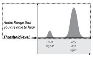
A Threshold level that is too low does not allow faint target signals to be heard.
