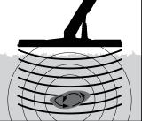
The magnetic field produced by a target is dependent on two target electrical characteristics:
