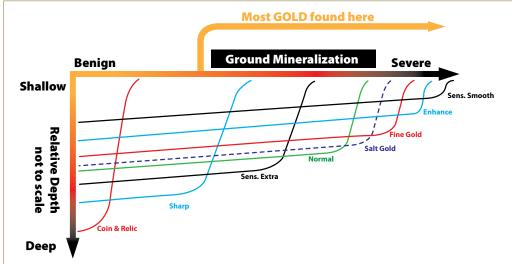
This easily memorized graph shows a simplified comparison between ground mineralization and relative Timing depth. It is not to scale and does not consider different size targets or show actual percentage of depth.
