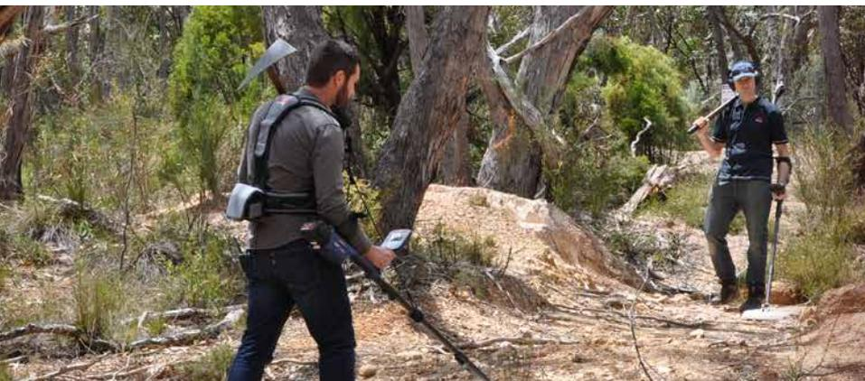
**“Once you set up the machine's ground balance with the yellow ferrite, it now tracks and stays balanced for the whole session.”**
