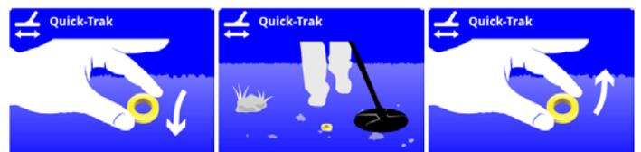
The ferrite ground balancing method is also explained on the multi-language reference card supplied with new detectors and accessory ferrites.
