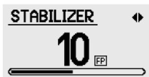
*Note: Regardless of which Audio Type is selected, the optimal position of the stabilizer is one number below the point where the threshold begins to chatter.*
