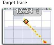
Target Trace displays many detections per second to offer greater visual detail of a target's identity. Multiple targets are displayed as coloured 'hot spots', or streaks, across the Detect screen dig. Eight Tone ID Profiles are turning everyone into experts. Choose to have on or off while detecting or during pinpointing.
